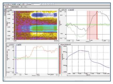
The above image displays representative data from a freely moving rat using Pinnacle's Wireless FSCV system with a 34 µm sensor. From top left to bottom right: heat map, voltammogram, current, background.
