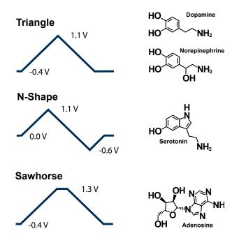
FSCV offers preprogrammed waveforms associated with commonly studied analytes. Custom waveforms can be easily uploaded and stored in a drop-down menu for quick selection.
